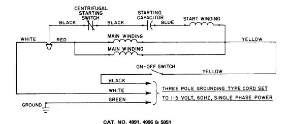
SCHEMATIC DIAGRAM FOR SINGLE PHASE GRINDERS
